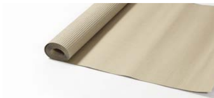
Uno Protect Non-mineral substrates / Wood substrates Footfall sound underlay Compressive strength up to 20,000 kg/m 2 Thickness: 2.2 mm
